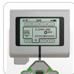
Port View with Gyro Sensor
